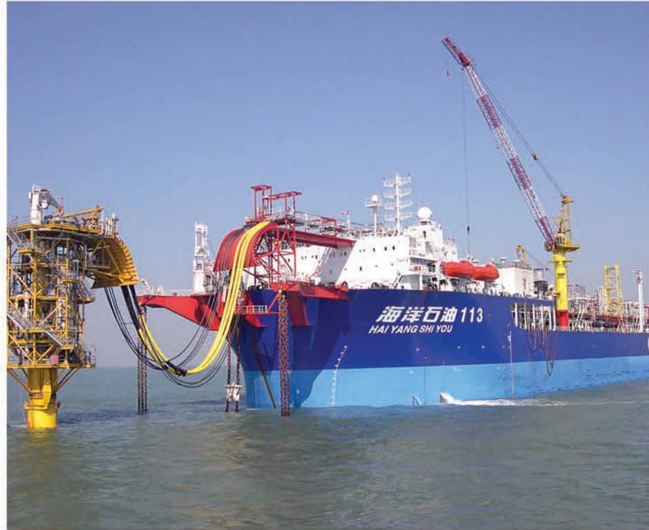
▼ 向中海油113号FPSO提供的高效油气处理设备 Provide High-efficiency Oil-dehydrate Treatment Equipment for CNOOC No.113 FPSO
