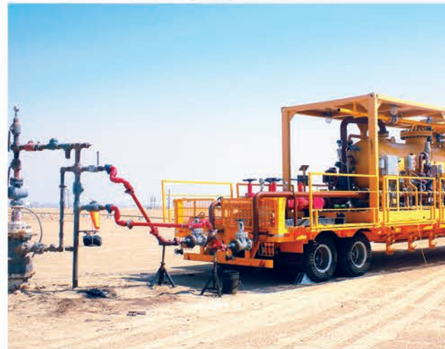
▼ 科威特WJO测试分离器 Kuwait Well Testing Equipment for WJO
