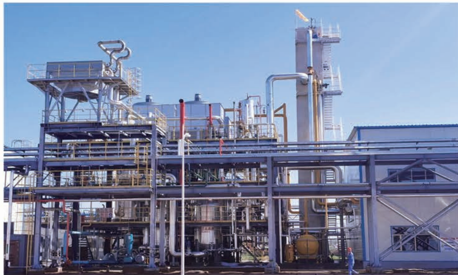
▲ 高纯度CO 2 (纯度≥99.996%, 回收率≥99%)生产装置, 可满足工业级和食品级应用要求 High-purity CO 2 (Purity ≥99.996%, Recovery Rate ≥99%) Production Device, Meeting The Requirements of Industrial Grade and Food Grade Applications
